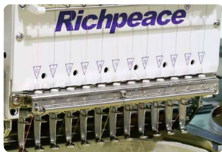
New upper thread holder: Reduce the thread breakage rate.
