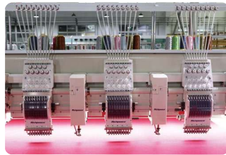
Latest thread clamping system and thread guiding tubes make it go more smoothly, lower thread breakage rate.
